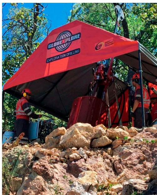
Figure 1 Mithril's drilling contractor, Globexplore Drilling with compact core rig in Mexico.
