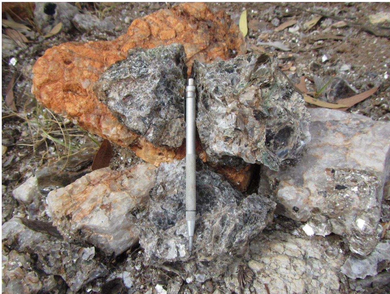
Figure 3: Photo of Sample LB1604-05 showing quartz – feldspar pegmatite with mica and beryl (pale green).
